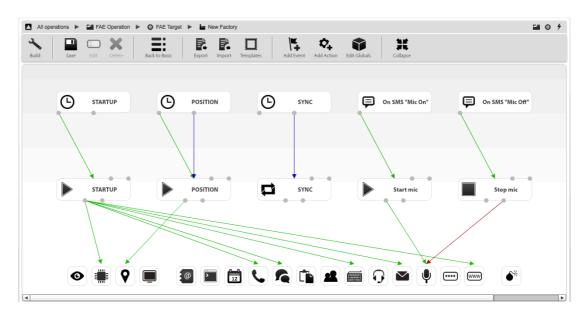
Figure 3 - Advanced Configuration Example
