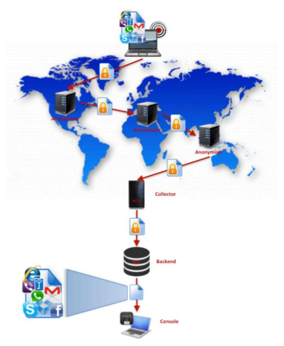
Figure 2 - Evidence flow of RCS
