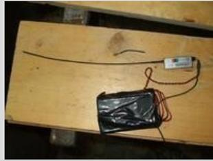
*The microphone without the tape and with the tip detached*
