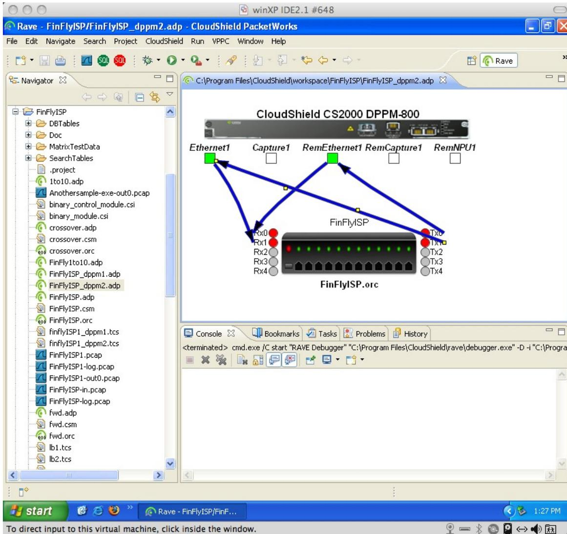
In addition to deploying the ADP files on the dual DPPM-800 system, there are two TCS configuration files that need to be deployed. In the project workspace these files are present and can be clearly identified as they have a .TCS file extension. This files should be used 'as is' and not modified.
